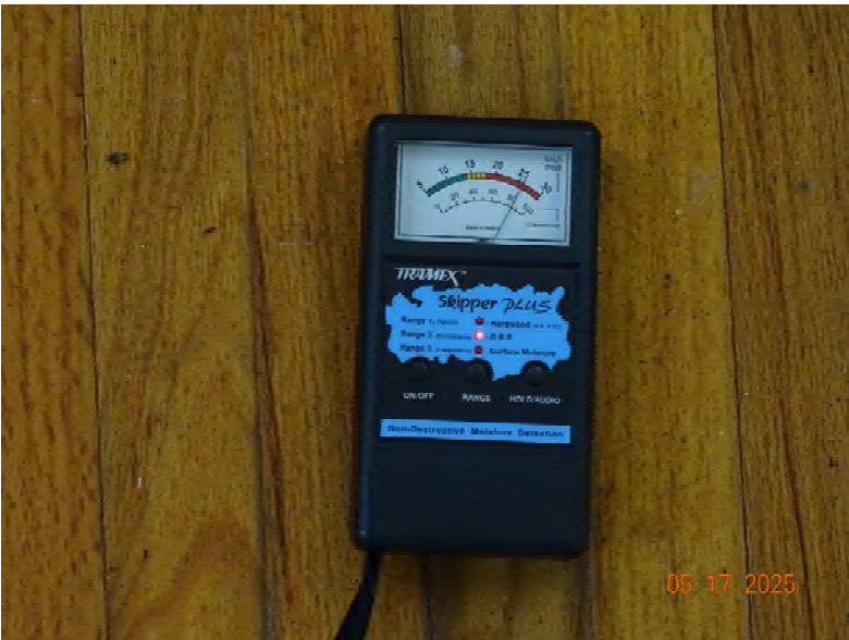
19 Moisture at floor
