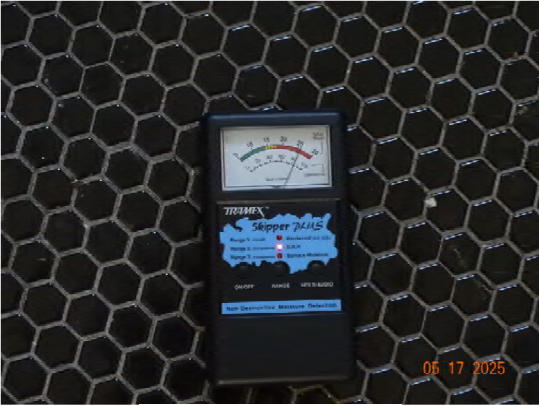
21 moisture at floor
