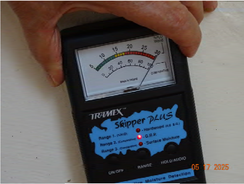
23 Moisture at wall
