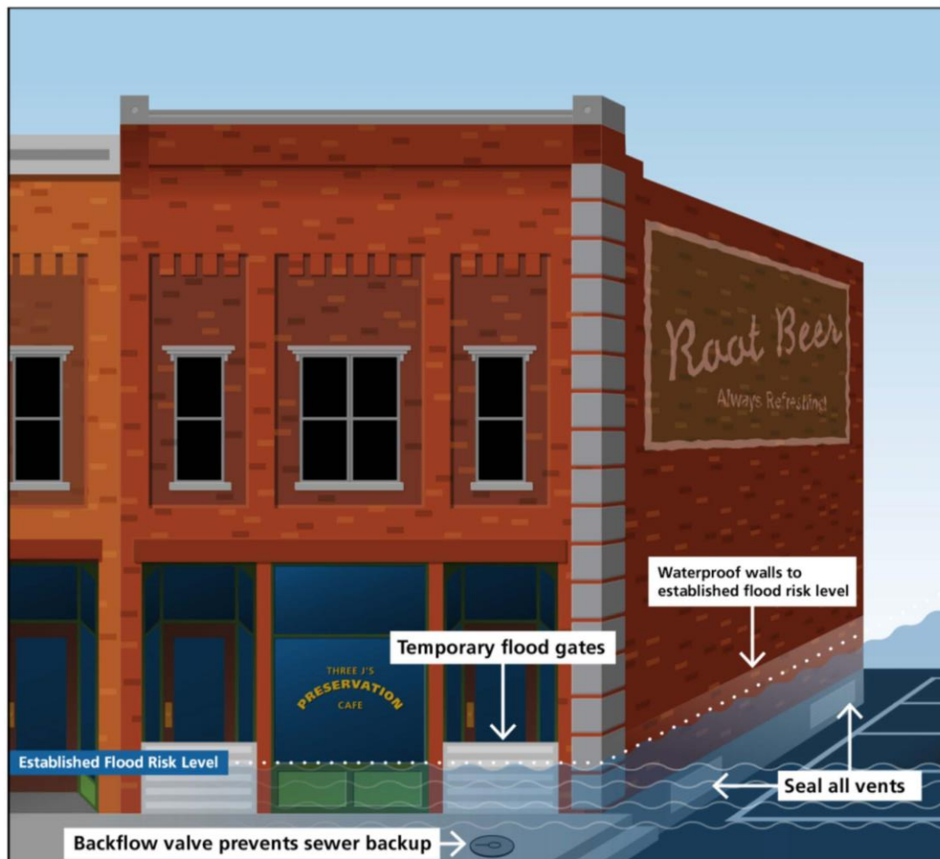
Figure 41. Methods for dry floodproofing, as illustrated by the National Park Service (NPS) in their Guidelines on Flood Adaptation for Rehabilitating Historic Buildings (2021).
